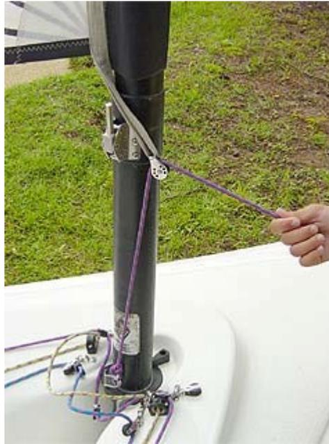
**Step 1:** Run the line attached to the mast just above the black bearing through the block attached to the foot of the main sail.
