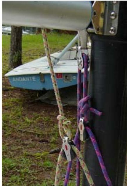
**Step 1:** Tie end of outhaul line (yellow in this photo) to the eye in the block using a bowline knot. Leave line as long as possible to get maximum travel during outhaul adjustment.
