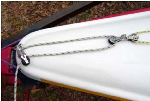
**Step 10:** Secure the tack line (maximum length 105") to the eye on the bow with a figure eight knot. Run other end through turning block , then back to bow and run through turning block.
