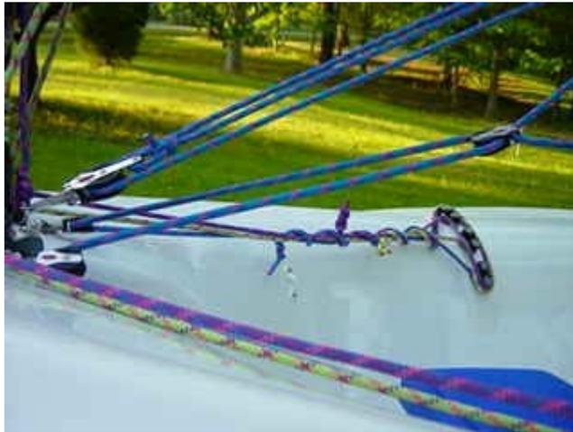
**Step 7:** Using a bowline, tie the remaining end of Vang line to the eye of the block located on the same colored Vang line that runs to either side of the Raider Sport cockpit.
