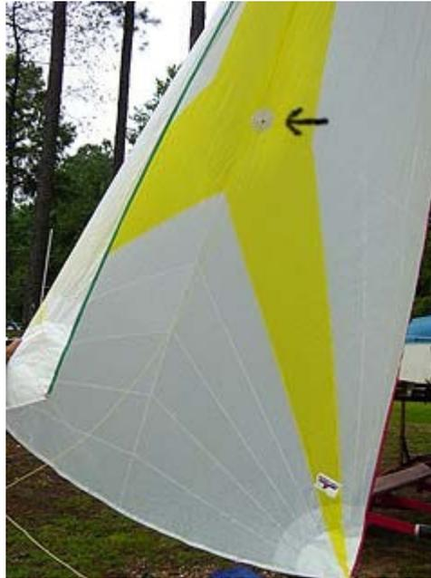
**Step 13:** With the spinnaker partially flying (held out) to the port side (left), locate the retrieval point (black arrow).
