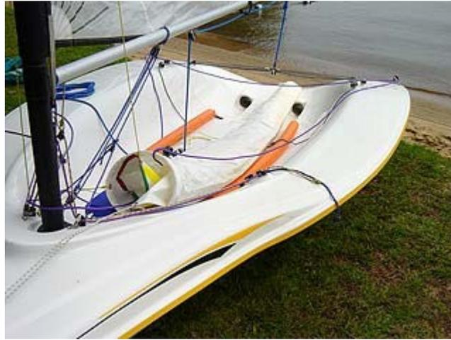
All that is left to complete the spinnaker rigging is to retrieve the spinnaker into the launch bag (ready for use) as shown in this photo. To retrieve, pull the spinnaker halyard from the same location as you did in Step 10. Only this time, pull from the aft forward. You may have to help the sail into the bag. Be sure the spinnaker sheet lines are not locked in the cam cleats.
