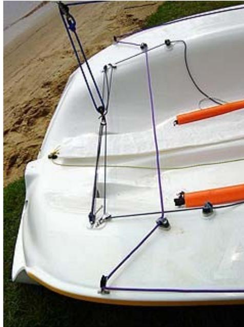
**Step 17:** Run the spinnaker sheet across the stern (back) of the boat. Be sure the sheet is run over all lines and equipment. Continue through the cam cleat on the starboard (right) side, then through the swivel block forward towards the mast.
