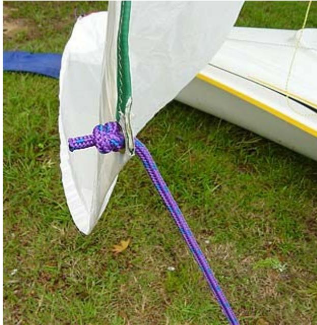
**Step 15:** Run one end of the spinnaker sheet through the grommet in the spinnaker. In this photo the spinnaker is flying on the port side (left), and the spinnaker sheet is stuck through the grommet back to front with a figure eight knot in the end.
