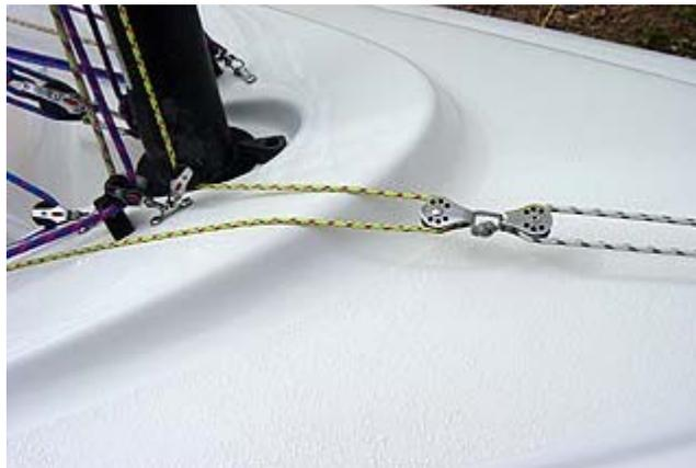
**Step 4:** Run the halyard through the turning block and back towards the back of the boat.
