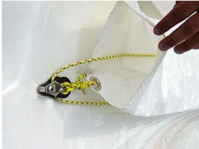
**Step 6:** Once the halyard is through the block, pull the halyard through the launch bag up to the front of the cockpit. The launch bag should be lying on the left side of the cockpit floor. Then tie the small end of the launch bag to the block as close as possible.
