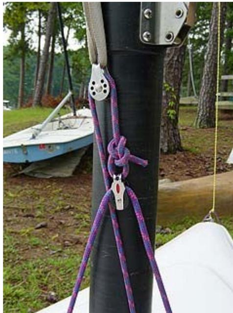
**Step 2:** Tie end of Vang line to eye in single block using a bowline knot. Try to get as close as possible to the first block attached to sail.
