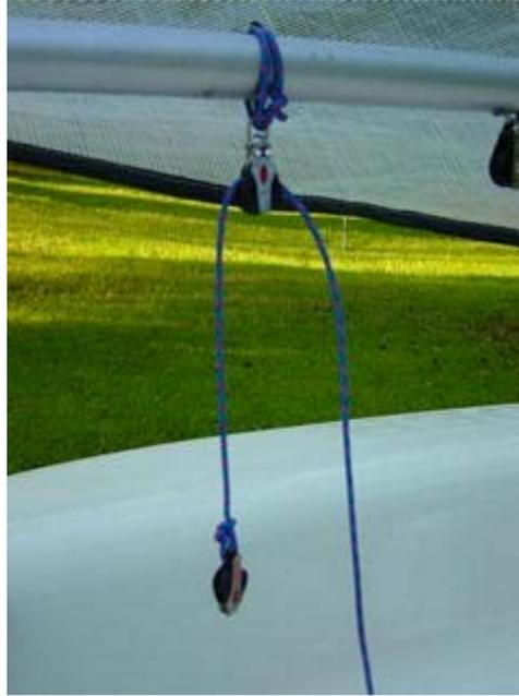
**Step 3:** Thread other end of Vang line into double block on boom.
