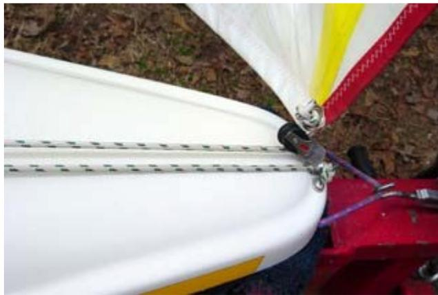
**Step 11:** Run tack line aft, make sure it is over the top of all control lines. Secure end to tack of spinnaker using a figure eight knot.
