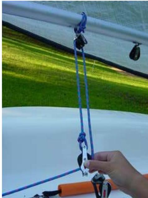
**Step 4:** Continue threading Vang line in a clockwise direction into single block.
