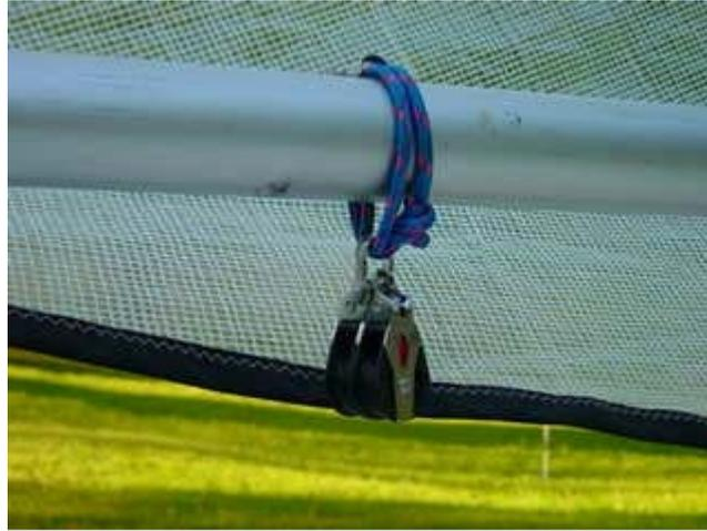
**Step 1:** Tie double block to boom using a square knot. Be sure line goes through eye on top of boom.
