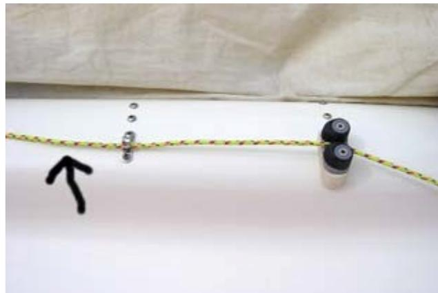
**Step 12:** Raise the spinnaker about half way by pulling the halyard towards the rear of the boat. The arrow in the photo shows where to pull from.
