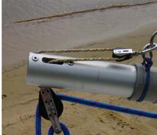
**Step 3:** At the opposite end of the boom the outhaul line exits from the turning block towards the sail around the hook ( in this photo the line goes through the optional pulley) and back to the grommet in the boom with a figure eight knot securing it in place.
