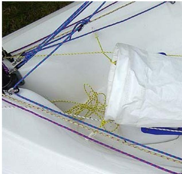
**Step 8:** This is how the launch bag looks from the port side (left) with the spinnaker halyard exiting the front of the launch bag.
