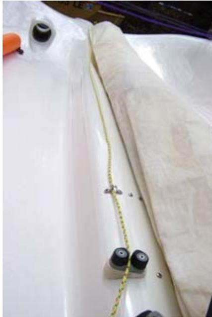
**Step 5:** Continues the halyard aft under the control lines, through the block attached to the hiking strap eye, through the cam cleat and the eye towards the back of the boat.
