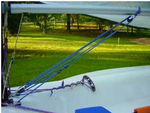
You have completed the installation process of the Boom Vang, this photo shows the completed setup. If yours does not look the same, please review the steps above. For storage undo shackle in Step 6 and bowline in Step 7. Keep lines running through blocks.
