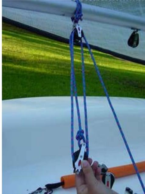
**Step 5:** Continue threading Vang line in a clockwise direction into the remaining position on the double block.
