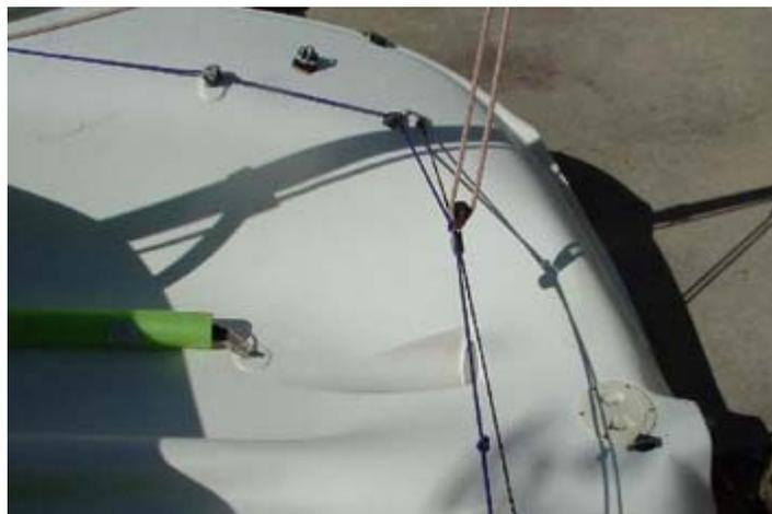
I tied two stopper knots 16" apart (8" ea. side of center) on the traveler control line. In 8 to 12 wind speed, the boat seemed to have same pointing ability with more power up wind. The laser sailors have been doing essentially the same thing for years. Works for them, works for us too!
