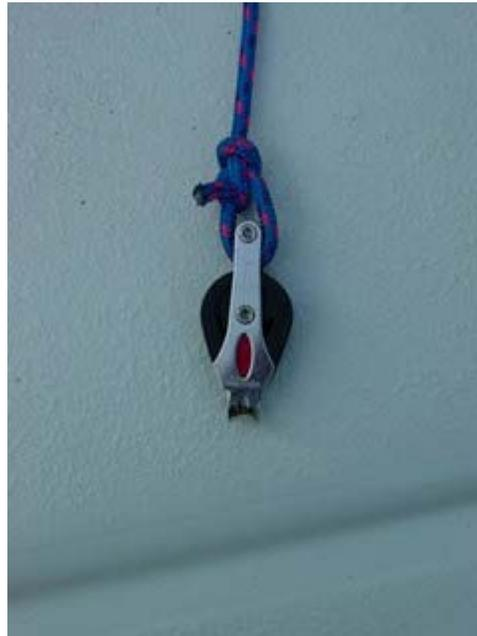
**Step 2:** Tie end of vang line to single block using a Bowline knot.
