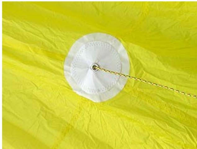
**Step 14:** Take the spinnaker halyard end that is coming out of the front of the launch bag and run it through the grommet in the middle of the retrieval point. Tie a figure eight knot on the back side as close to the end as possible to keep the halyard from pulling back through. Be sure that the halyard is run above all lines as it exits the launch bag and attaches to the retrieval point.
