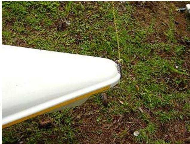
**Step 2:** Temporally tie one end of the spinnaker halyard to the bow.
