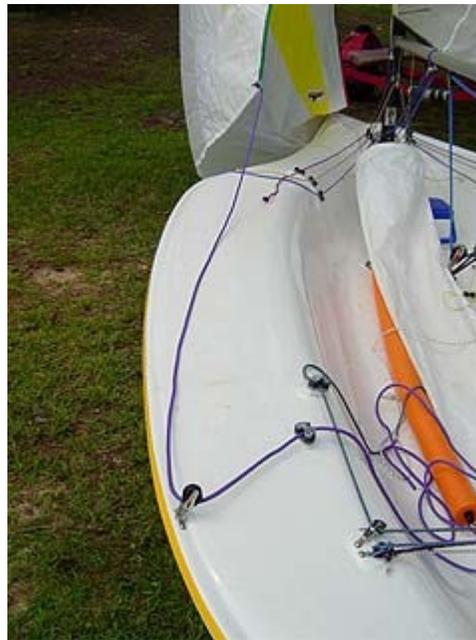
**Step 16:** Take the other end of the spinnaker sheet and run it aft along the port side (left) of the boat, through the swivel block, and through the cam cleat.
