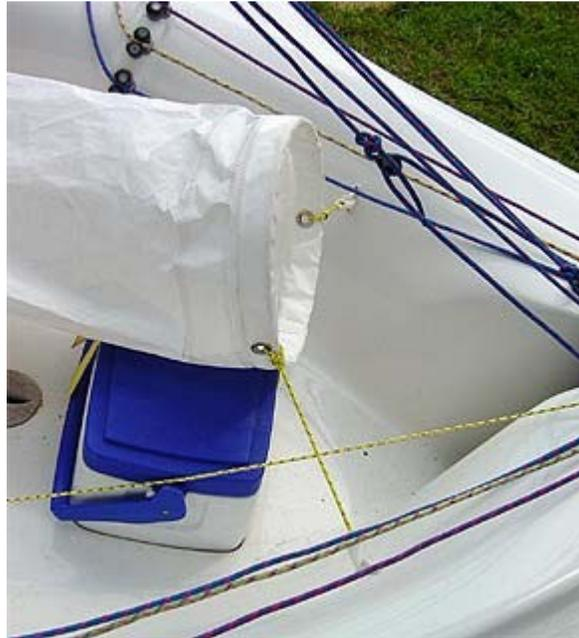
**Step 7:** Secure the launch bag to the sides of the cockpit. The short line goes to the port side (left). Be sure the lines are run under all control lines.
