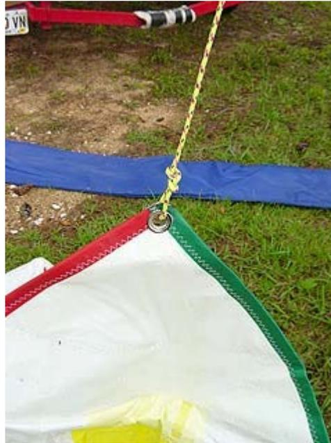
**Step 9:** Untie the end of the spinnaker halyard that you temporarily attached to the bow. Using a bowline attach this end to the top of the spinnaker.
